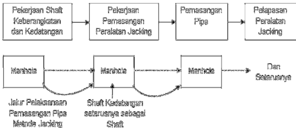
Gambar 41 Tahap Pelaksanaan Metode microtunneling/jacking
